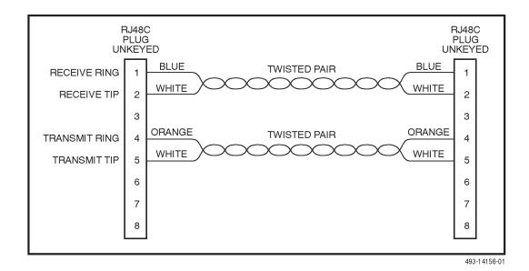
Figure D-1. T1 Line Interface Cable, RJ48C-to-RJ48C
